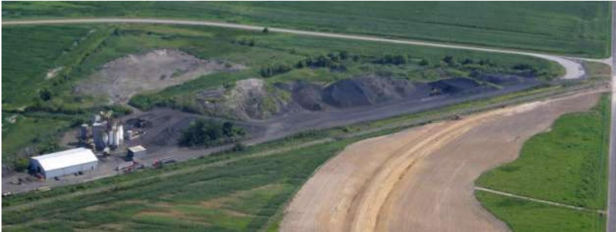
U.S. Minerals uses the bottom ash from Coffeen Power Station for making construction materials. Coal ash is stored in large piles at the industrial site, a half mile north of Coffeen Power Station. The piles of coal ash do not have liners, covers, windbreaks, or silt fences to prevent erosion and release of pollutants to air and water.
