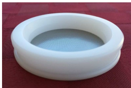
Figure 1. Filter cassette (filter not shown)
